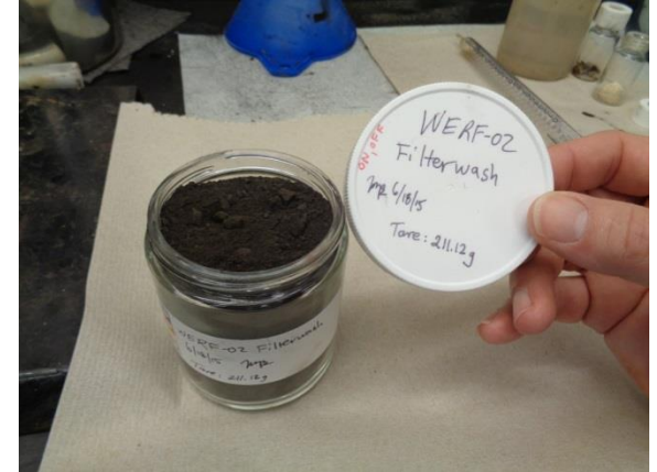
Solids from filter vessel
