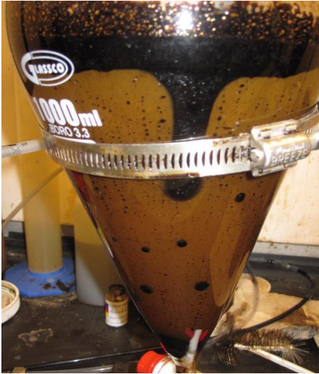
HTL steady state liquid effluent
