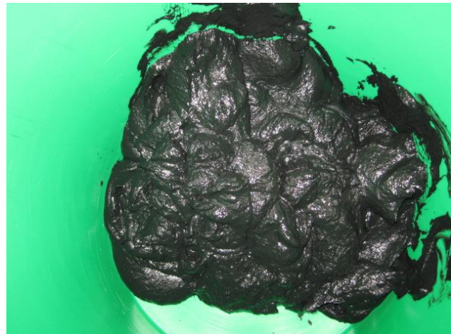
Post-digester (16.4 wt % solids)
