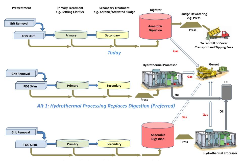
Alt 2: Hydrothermal Eliminates Digester Sludge
