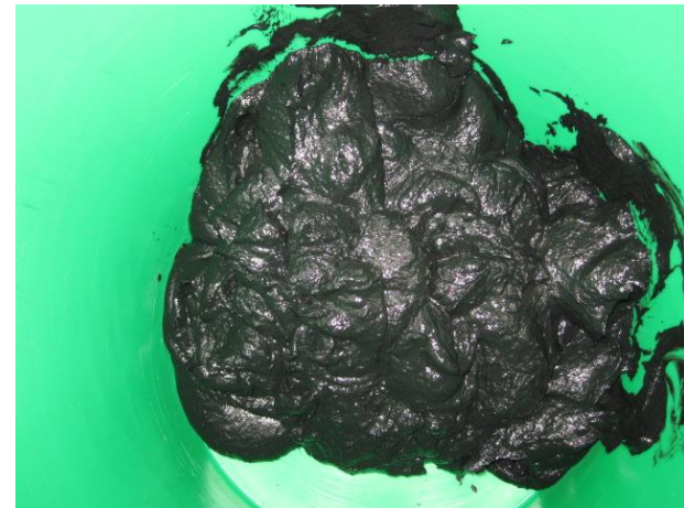
Post-digester (16.4 wt % solids)
