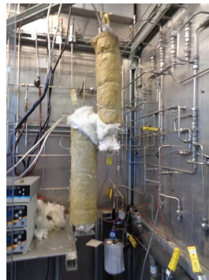
Precipitator and Reactor
